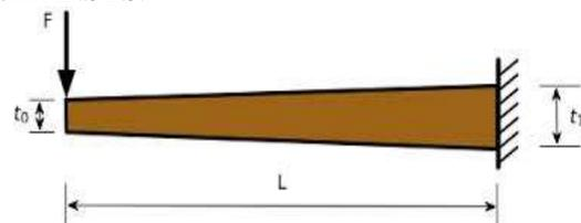
Fig 1. Tapered cantilever Beam
