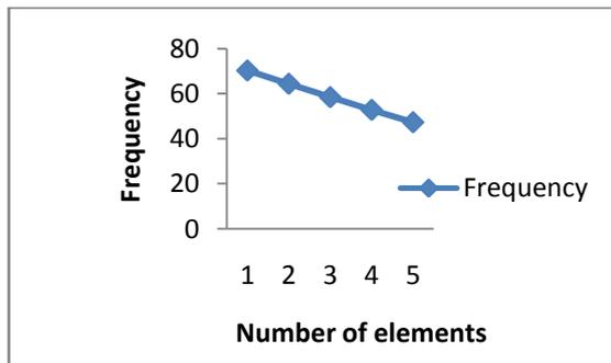
Figure 1. Convergence of fundamental natural frequency for Cantilever beam.
